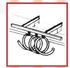
Attention: all the power-driven reels are equipped with upwards / downwards electric adjustment safety stops. In order to supply electricity to the power-driven reels it necessary feeding line mod. LMF
